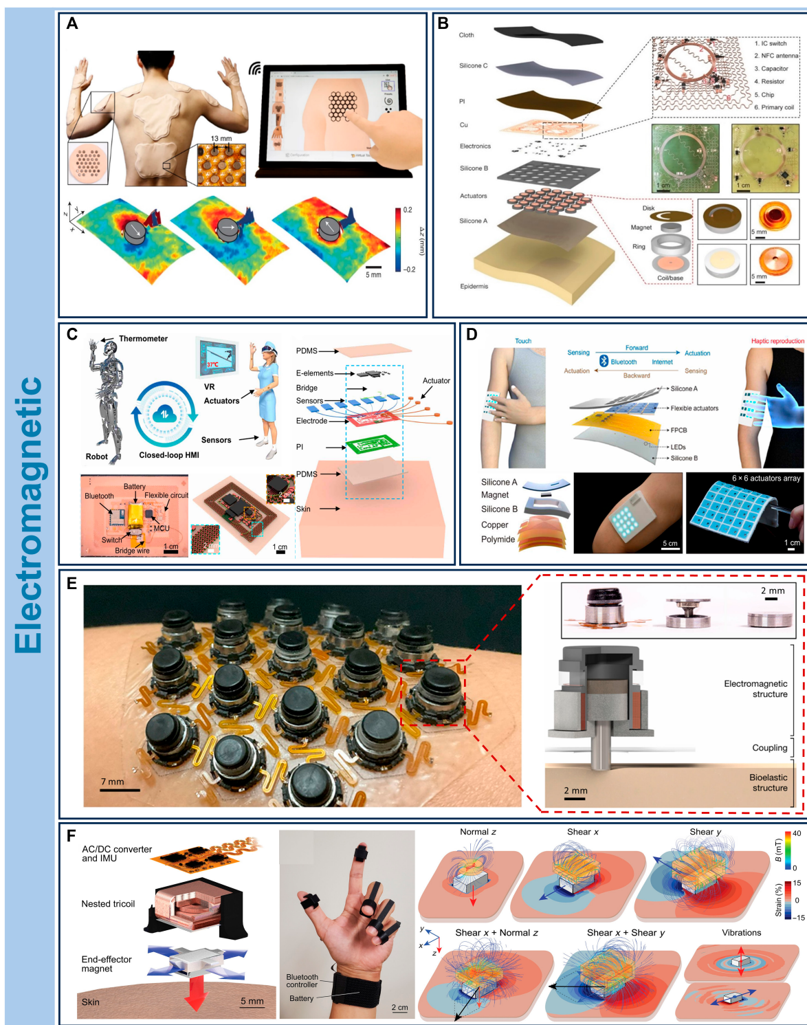
Fig. 5. Electromagnetic haptic wearable systems. Representative platforms for electromagnetic-based haptic feedback. (A) High-density hexagonally tiled actuator array integrating up to 147 eccentric rotating mass (ERM) units for distributed haptic feedback across multiple body regions. Copyright 2022, Springer Nature [19]. (B) Exploded schematic of a large-scale, wireless electromagnetic actuator array for flexible skin interfaces. IC, integrated circuit. Copyright 2019, Springer Nature [22]. (C) Closed-loop electronic skin (e-skin) enabling full-body motion capture and real-time haptic interaction in virtual environments. MCU, microcontroller unit. Copyright 2022, AAAS [25]. (D) Self-sensing, soft electromagnetic actuator array forming a reproducible and conformal haptic e-skin platform. LEDs, light-emitting diodes. Copyright 2022, AAAS [20]. (E) Bistable haptic interface leveraging skin elasticity as an energy storage medium to enable multimodal tactile stimulation, including pressing, vibration, and torsional feedback. Copyright 2024, Springer Nature [93]. (F) A full freedom-of-motion (FOM) actuator system delivering programmable normal, shear, and torsional forces for immersive haptic feedback and spatial navigation. IMU, inertial measurement unit. Copyright 2025, AAAS [94]. Copyright as indicated; all reproduced with permission.
