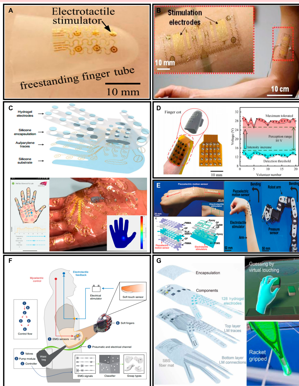
Fig. 2. Representative wearable electro-haptic systems. (A) Ultrathin fingertip sleeve with electro-tactile stimulation enabled by silicon nanomembrane diodes for circuit multiplexing. Copyright 2012, IOP [34]. (B) Multifunctional epidermal platform integrating electro-haptic output with electromyography, strain, and temperature sensing for motion management. Copyright 2016, Wiley [35]. (C) Personalized high-density wireless electro-tactile system (WeTac) with dynamic stimulation threshold mapping. Copyright 2022, Springer Nature [40]. (D) High-frequency AC electro-haptic device enabling low-voltage operation and high-resolution feedback across 25 electrodes. Copyright 2022, AAAS [41]. (E) Transparent, stretchable system integrating electro-tactile feedback and piezoelectric sensing for bidirectional human–robot interfaces. Copyright 2014, Wiley [42]. PMMA, polymethyl methacrylate; SWNTs, single-walled carbon nanotubes; AgNW, silver nanowire; PDMS, polydimethylsiloxane; GP, graphene; PLA, polylactic acid. (F) Neuroprosthetic hand with myoelectric control and real-time electro-tactile feedback delivered to the residual limb. Copyright 2023, Springer Nature [26]. (G) Breathable, textile-based electro-haptic system with 128 stimulation pixels for extended virtual reality interaction. SBS, poly(styrene-block-butadiene-block-styrene); LM, liquid metal. Copyright 2024, AAAS [45]. Copyright as indicated; all reproduced with permission.
